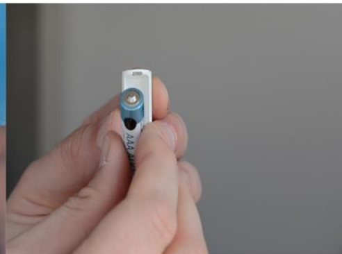
2. Install AAA battery into Tethercell adapter.
